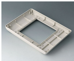
B4044707 Bottom part M flat, version I ABS (UL 94 HB) off-white RAL 9002 225x165x25,5mm IP 54 opt.
