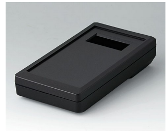
A9073219 DATEC-MOBIL-BOX S, Vers. II ABS (UL 94 HB) black RAL 9005 152x83x33,5mm IP 65 opt.
