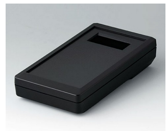
A9073419 DATEC-MOBIL-BOX S, Vers. IV ABS (UL 94 HB) black RAL 9005 152x83x33,5mm IP 65 opt.
