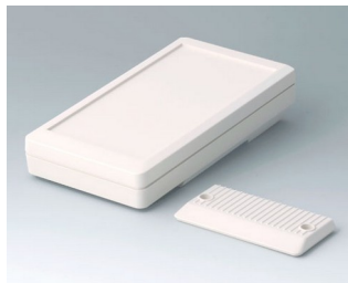
A9073107 DATEC-MOBIL-BOX S, Vers. I ABS (UL 94 HB) off-white RAL 9002 152x83x33,5mm IP 65 opt.
