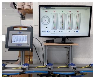
Monitoring system for cleaning nozzles
