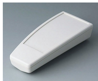
A9067117 SMART-CASE L, Vers. II ABS (UL 94 HB) off-white RAL 9002 140x62,7x30,5mm IP 65 opt., IP 40
