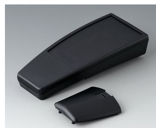
A9068209 SMART-CASE XL, Vers. I PMMA (IR) (UL 94 HB) black RAL 9005 168x74,4x35,4mm IP 40
