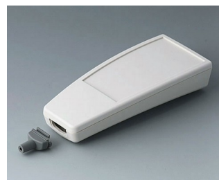
A9068137 SMART-CASE XL, Vers. IV ABS (UL 94 HB) off-white RAL 9002 168x74,4x35,4mm IP 65 opt., IP 40
