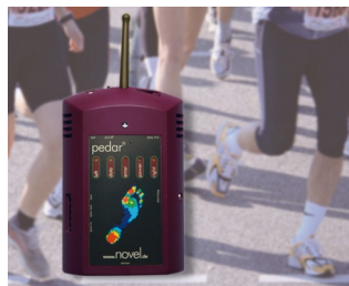
Dynamic pressure measuring between foot and shoe
