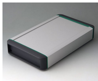
B3407031 SMART-TERMINAL 240 Aluminium AlMgSi 0,5 matt anodised 282x170x50mm IP 54
