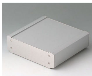
B3407013 SMART-TERMINAL 160 Aluminium AlMgSi 0,5 matt anodised 164x170x50mm
