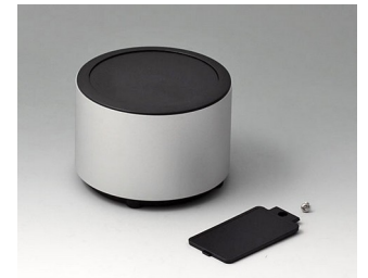
ER106059 SYNERGY R100 Aluminium AlMgSi 0,5 matt anodised ø100x70mm IP 40
