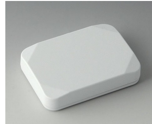
B1824117 MINI-DATA-BOX E50, flat ASA+PC (UL 94 V-0) traffic white RAL 9016 70x50x15mm IP 65 opt., IP 40
