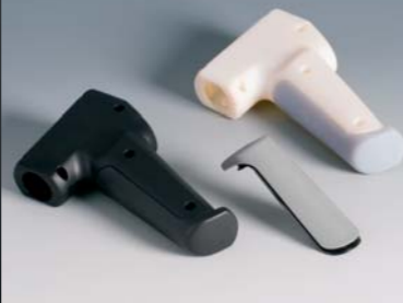
STL prototype 1 and part 7 with double injection technique
