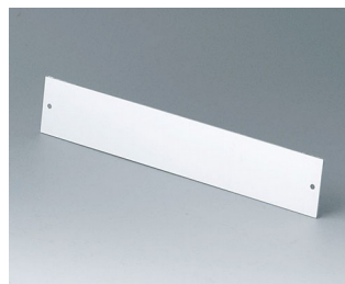
A9185001 Front panel Aluminium matt anodised 200x35x1.5mm
