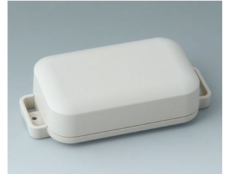
C3206207 EASYTEC 100 ASA+PC (UL 94 V-0) off-white RAL 9002 121x62x31mm IP 65 opt., IP 40
