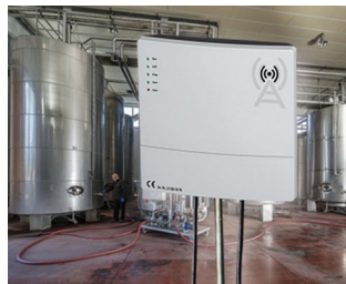
Gateway for the automation of production plants
